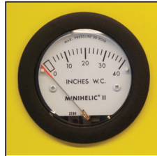
Gauge tells you when to clean filters
